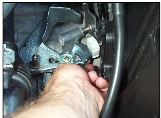
Figure 42 - Slide the Side To Side Bracket towards the Driver Side of the Car
