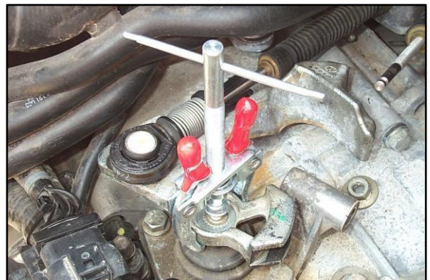
Figure 49 - Using a Battery Terminal Puller to Remove the Chrome Bracket from the Selector Shaft
