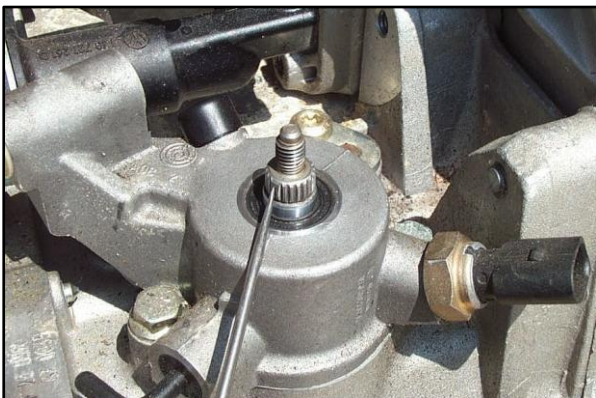
Figure 48 - Remove the Chromed Shift Bracket from the Splined Selector Shaft of the Transmission
