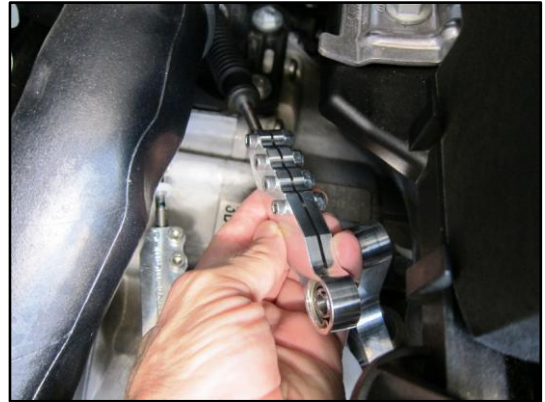
Figure 74 - Make Sure One More Time That the Side To Side Cable End Slides Freely
