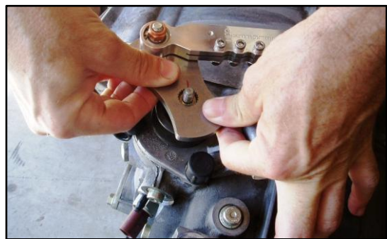
Figure 63 - Shift Bracket Will Push Pretty Easily Onto the Selector Shaft
