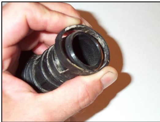
Figure 8 - Squeezing Where the Serrations Are On the Outer Ring
