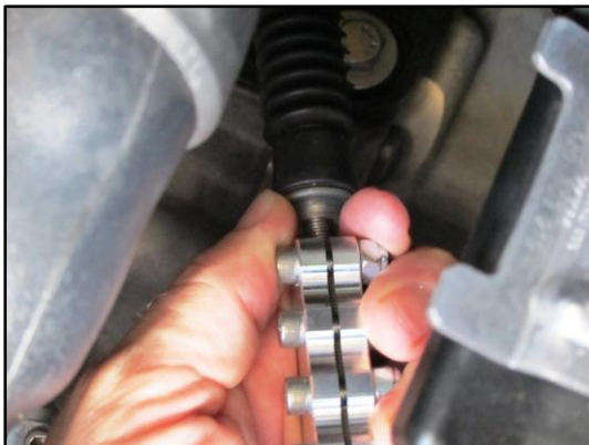
Figure 90 - Remove the Slack from the Side to Side Cable by Gently Pulling the Shift Cable Out of the Cable End
