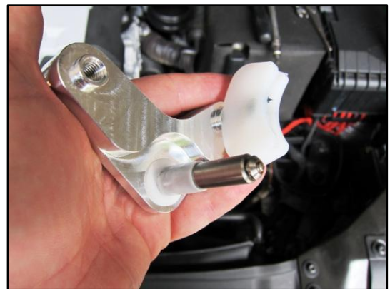
Figure 67 - Slide One of These White Plastic Bushings onto the Silver Side To Side Bracket Pivot Pin
