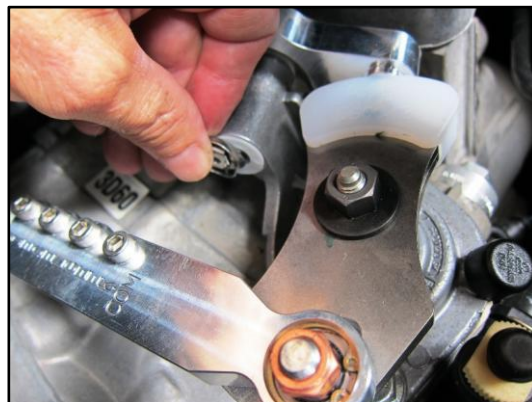
Figure 70 - As You Are Putting the Side To Side Lever In, Engage the Slot of the White Plastic Slider with the Front to Back Bracket
