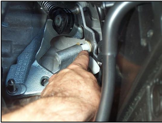
Figure 43 - Two Round White Plastic Pivot Bushings
