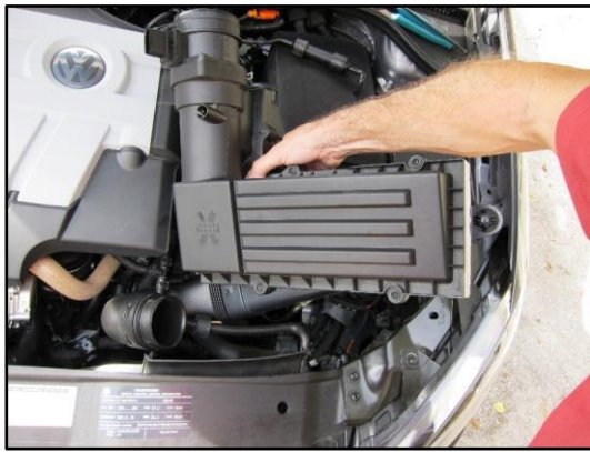
Figure 29 - Maneuvering the Intake Snorkel Underneath
