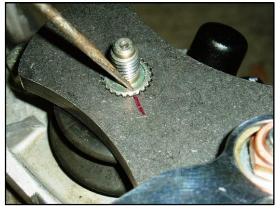
Figure 61 - "Keyway" Or Two Joined Splines on the Selector Shaft on the Transmission
