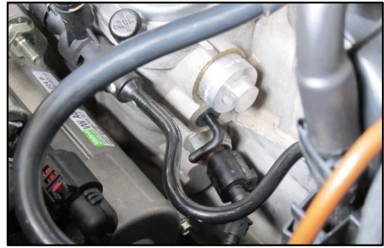
Figure 82 - Black Plastic L Shaped Lever Just Above the Electrical Plug
