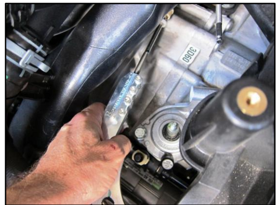
Figure 59 - Slide the front/back lever's aluminum cable end onto the shift cable closest to the engine
