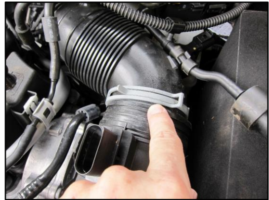
Figure 19 - Set the Clamp Just Behind the Normal Clamping Position
