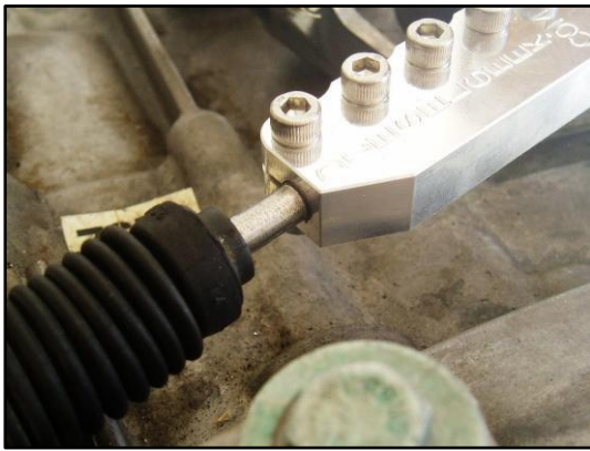
Figure 60 - Make Sure the Cable Can Be Inserted Into the Cable End Until the Threads Disappear Inside the Cable End
