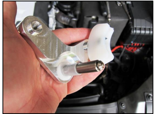
Figure 44 - Transfer the Bushing to the New Dieselgeek Side To Side Bracket Side To Side Bracket
