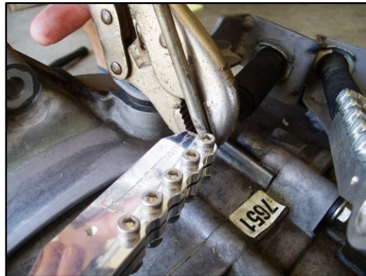
Figure 98 - If The Cable End Still Does Not Want To Slide Off You Can Clamp A Vice-Grip Next To A Fully Loosened Cable End And Pry It Off With A Flat Blade Screwdriver
