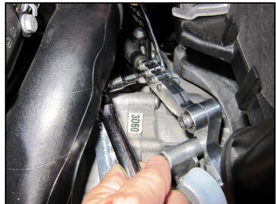
Figure 91 - Tighten Only the 2nd Allen Screw on the Cable End with a 4mm Allen Wrench and a Box End 3/8 Wrench to Hold the Lock Nut
