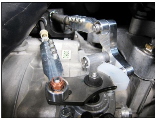
Figure 78 - Shifter Parts Are Now Installed
