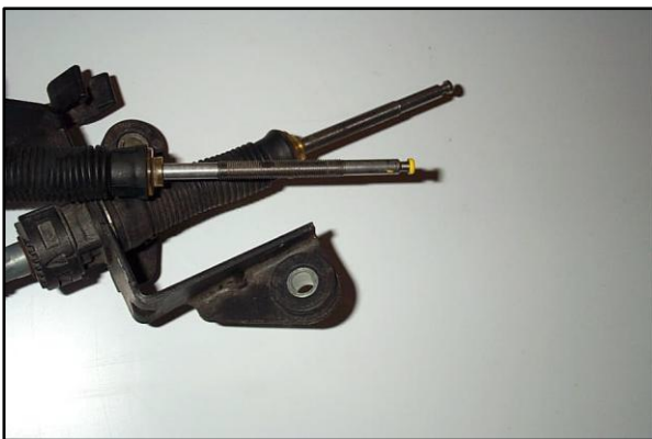
Figure 54 - Pull Back the Front to Back Cable Rubber Boot (If Present) and Plastic Ring to Expose All Threads of This Cable
