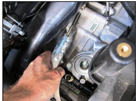
Figure 51 - This Bracket's Cable End Should Be Slid Onto the Cable Closest To the Engine
