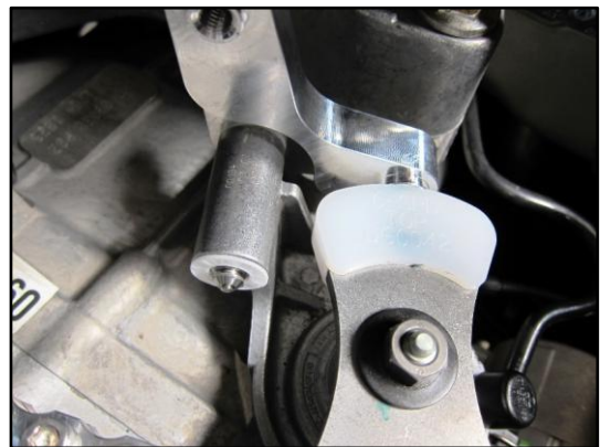
Figure 69 - Make Sure That The Other White Plastic Bushing Is In Place On The Other Side Of The Tube As You Are Sliding The Pivot Pin Through The Hole.
