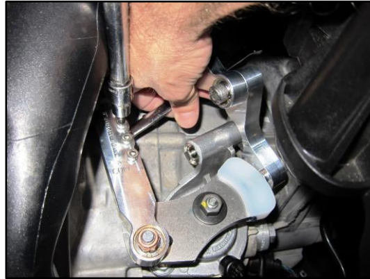
Figure 89 - Tighten a Single Allen Screw on the Front to Back Cable End Only
