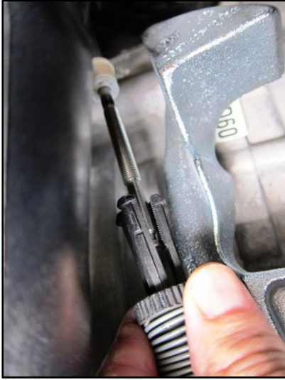
Figure 39 - Slide the Cable Ends Off
