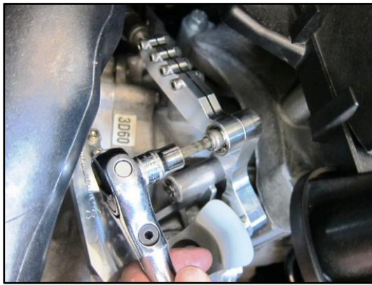
Figure 77 – Once the Socket Is In Place, Tighten the Allen Screw with a 6mm Allen Socket
