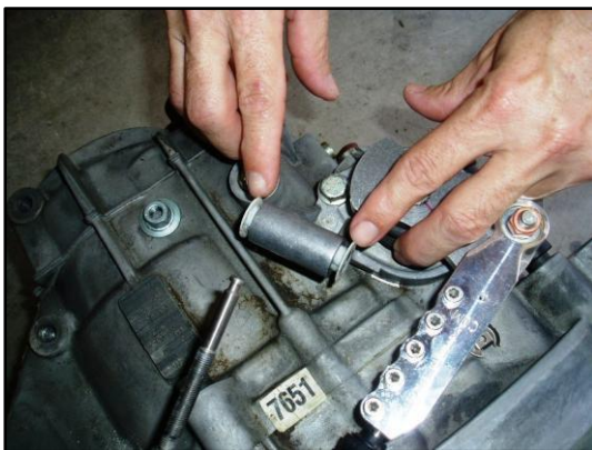
Figure 66 - Two Round White Plastic Bushings in the Aluminum Pivot Hole on the Transmission
