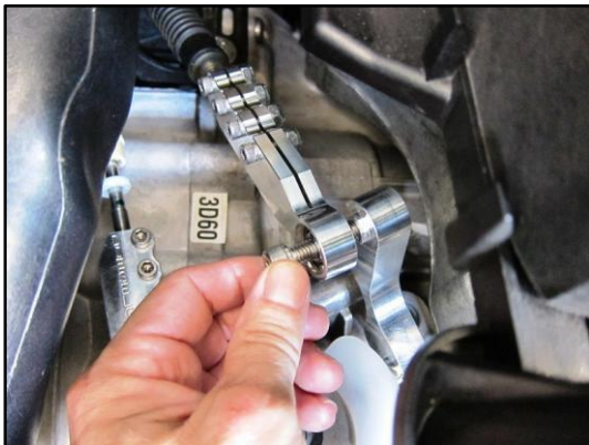
Figure 75 – Once the Cable End Is On the Cable, Thread in By Hand the 8mm Allen Bolt Supplied In the Parts Kit
