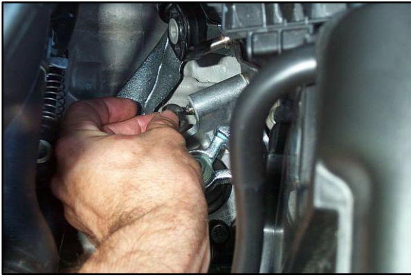
Figure 31 - Remove the Shiny Metal Clip for the Silver Side to Side Shift Bracket
