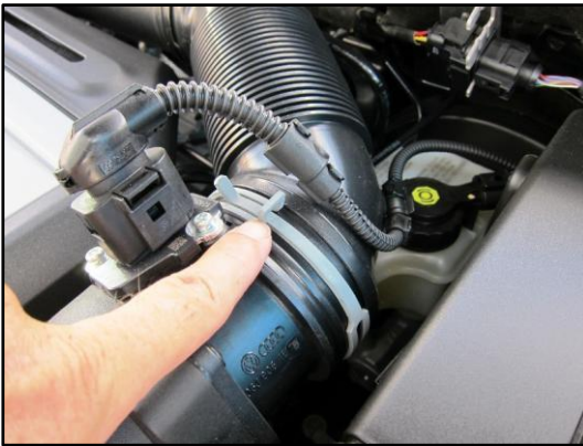
Figure 18 - Remove the Light Gray Spring Hose Clamp Holding the Flexible Air Pipe
