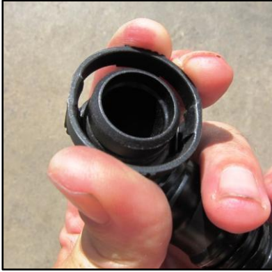
Figure 25 – Pinching the Two Ribbed Areas
